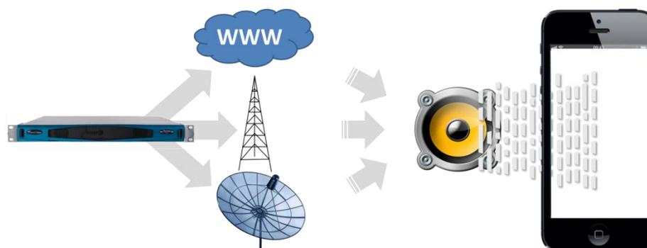
The Microvideo inserter, inserts the Intrasonics data which is then decoded by the smartphone, making the smartphone a completely interactive 2<sup>nd</sup> screen
